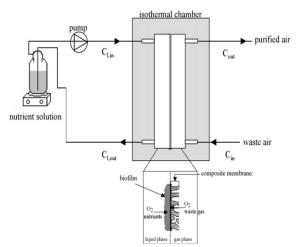
Fig: 1. Membrane bioreactor for removal of waste gas [2]
