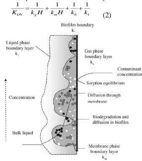
Fig: 2. Mass transfer resistance in a biofilm attached on a flat membrane
